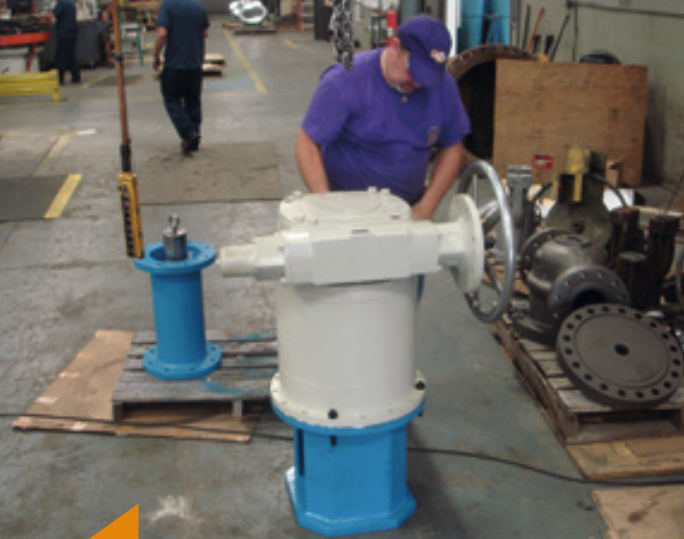
IM-50 (50 T DOWN FORCE) AT ASSEMBLY
